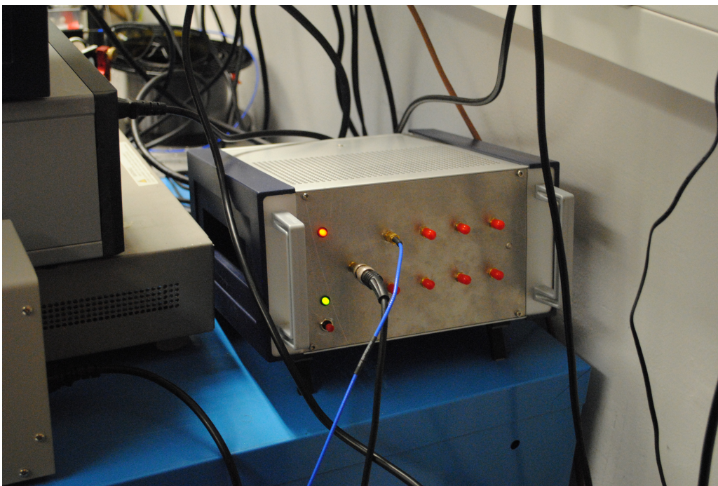
fig. 3.2: The green led acts the same as the "ACT" led on the Raspberry Pi itself, so it indicates if the Pi is on. The red led indicates that the entire board is attached to power. The button below the green led is for turning of the Pi.
